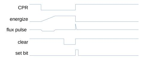
Note how the "clear" signal, which is required to clear the data latches before setting the "1" bits, precedes the end of the CPR (energizing) signal, such that it does not conflict with the pulses that set "1".
