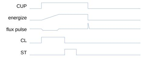
So, the question is how can the "normal" pulse generated at the end of the CUP signal be used to set latches if those are only enabled during the ST signal which precedes that event. I've been over the schematics, and even compared them to hand-drawn schematics I made in 1984 (before official schematics were publicly available). Everything suggests that my interpretation of the signals timing and usage is correct.
