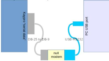
Connecting to a PC that has a legacy serial port:
