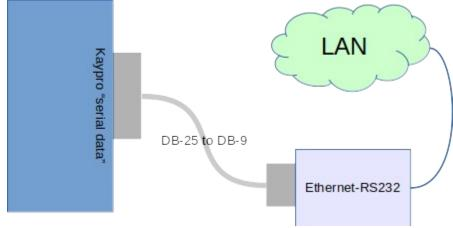
The configuration of the Ethernet-RS232 device is beyond the scope of this document. Attaching a terminal program over the LAN is also beyond the scope of this document. A gender adapter may be required, or even a null-modem, depending on the model of Ethernet-RS232 device.
