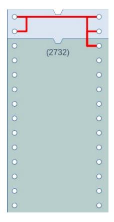
Using a socket adapter requires that the 28C64 be programmed with the image in the upper half (1000H-1FFFH), or else replicated in both halves.
